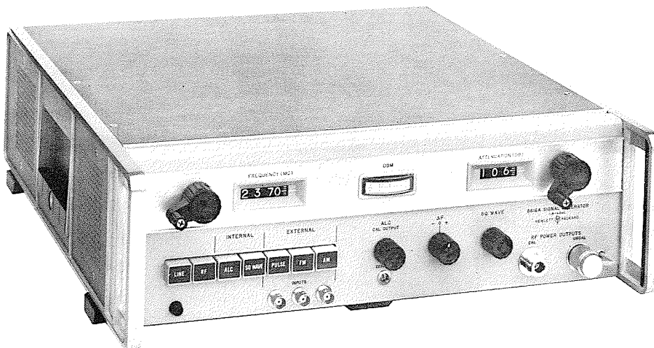
Figure 1-1. Model 8616A Signal Generator (The Model 8614A is exactly the same in physical construction)
